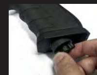
Turn the knob clockwise immediately to release the striker of the cap, Co2 will come out and fill the gun automatically.
